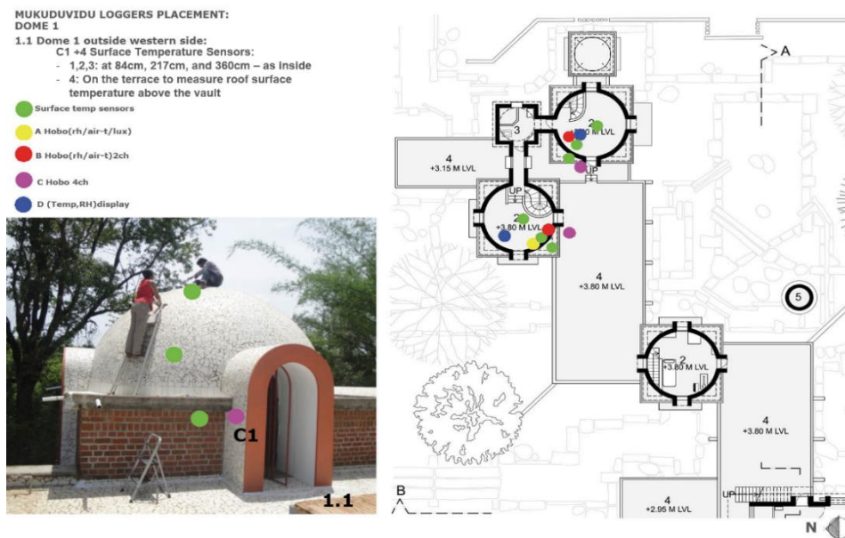
Figure 32 Placement of loggers on the first dome – top view
