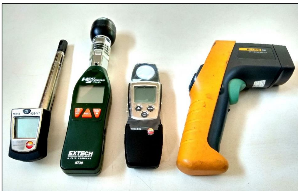
Figure 12 Handheld measurement instruments: Testo 405-V1 Anemometer, Extech HT30 Heat Stress Meter, Testo 540 Lux Meter, and Fluke 561 – IR Thermometer respectively
