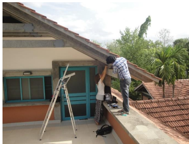
Figure 24 Installation of terracotta surface temperature sensor, logger C3
